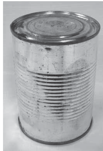
Pitted rust or leaking
