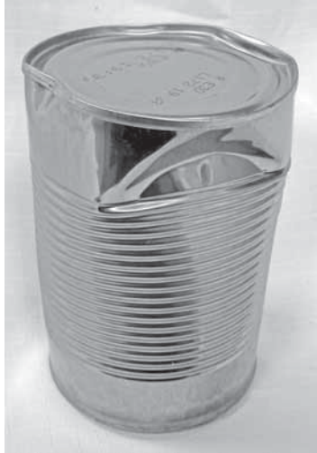
Dented at junction of side and end
